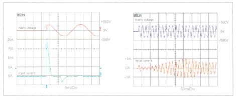
Figure 2. Inrush current behaviour, left conventional, right Maxpower
